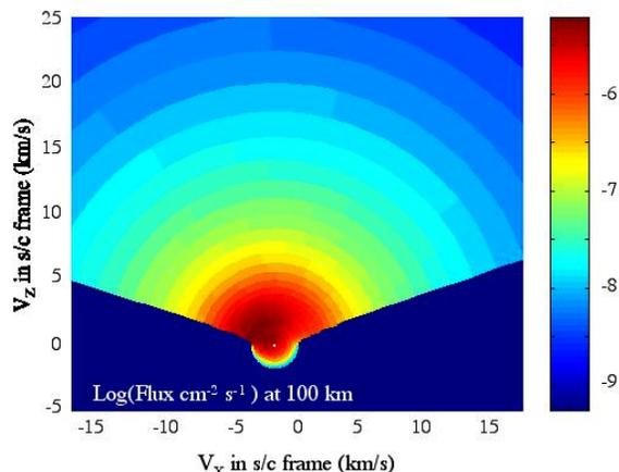
Fig 2. Log of neutron leakage flux at 100 km altitude, for FAn at 300 K.
