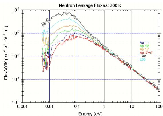
Fig. 1. Neutron leakage flux as a function of energy for six compositions
